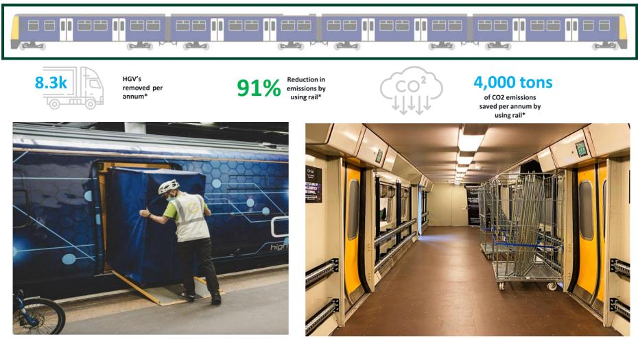
Handler loading a roll cage onto a converted passenger train for high-speed logistics
