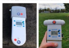
Figure 2.1: Aeroqual Series 500 handheld air quality sensors with \text{NO}_2 and \text{O}_3 sensor heads attached (right).
