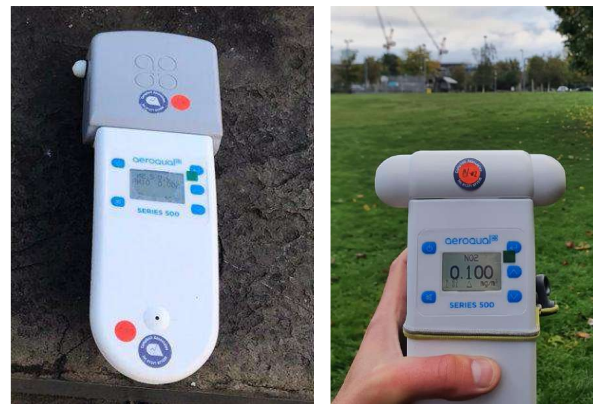
Figure 2.1. Aeroqual Series 500 Monitor Base (left) and with \text{NO}_2 and \text{O}_3 Sensor Heads attached (right).
