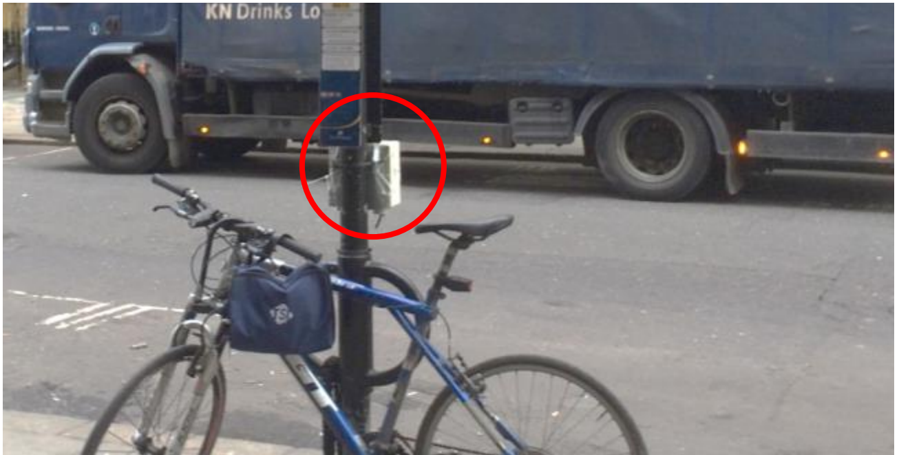
Figure 2 Placement of microAeth fixed to sign pole in weather proof box
