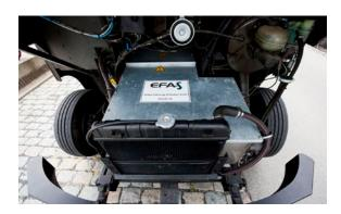
to retrofit the vehicles with an electric drive train and batteries. The converted vehicle has a payload of 3 tonnes and a range of approximately 100km, comfortably exceeding their average daily urban usage.
