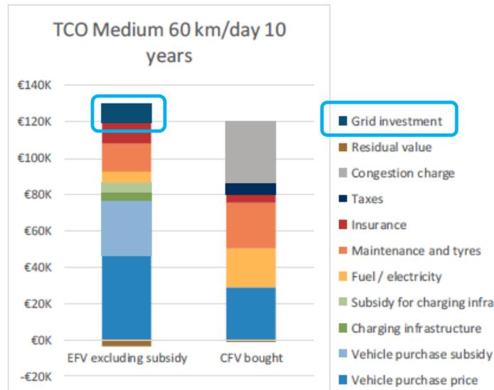
Figure 2. Total Cost of Ownership EFV vs CFV for a 3.5-7.5 tonne freight vehicle. Source: FREVUE (2017a)
